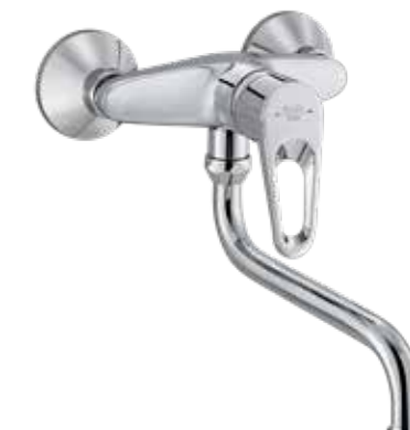
RAK30008 Wall mounted single lever sink mixer DN 15 ceramic cartridge-K35 swivelling (185°) spout l = 200 mm aerator M 22 x 1 flow class A S- unions 1/2 X 3/4 inch European standard- EN 817
