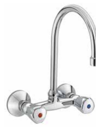
RAK35001SU Dual controlled wall mounted sink mixer DN 15 swivel U spout aerator M22 x 1 flow class A S- unions 1/2 inch x 3/4 inch European standard- EN200
