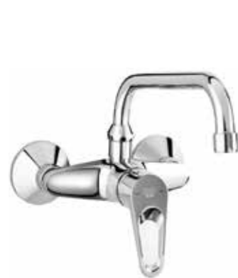
RAK30029 Wall mounted single lever sink mixer DN 15 ceramic cartridge-K35 swivelling (185°) spout l = 230 mm aerator M 22 x 1 flow class A S- unions 1/2 X 3/4 inch European standard - EN 817
