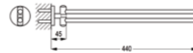
RAK21012 Double towel bar adjustable with adjustable two arm wall fastening with screws and dowels
