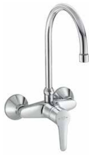
RAK10028SU Wall mounted single lever sink mixer DN 15 ceramic cartridge-K35 swivelling (185°) U spout l = 186 mm aerator M 22 x 1 flow class A S- unions 1/2 X 3/4 inch European standard- EN 817
