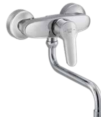
RAK11009 Wall mounted single lever sink mixer DN 15 ceramic cartridge-K35 swivelling (185°) spout l = 200 mm aerator M 22 x 1 flow class A S- unions 1/2 X 3/4 inch European standard- EN 817
